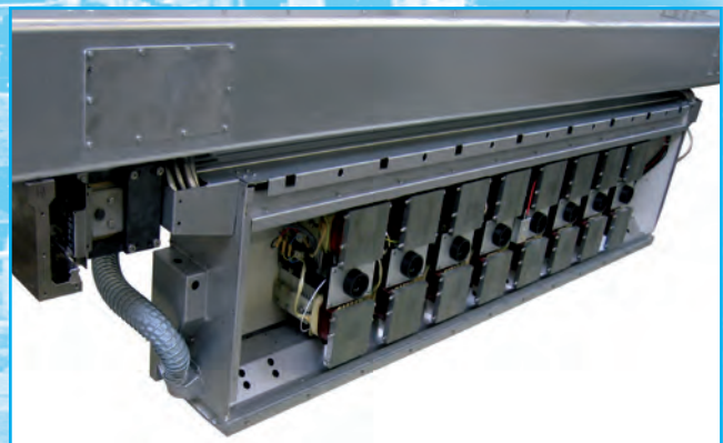
Inside of the housing (sensors and actuators)
