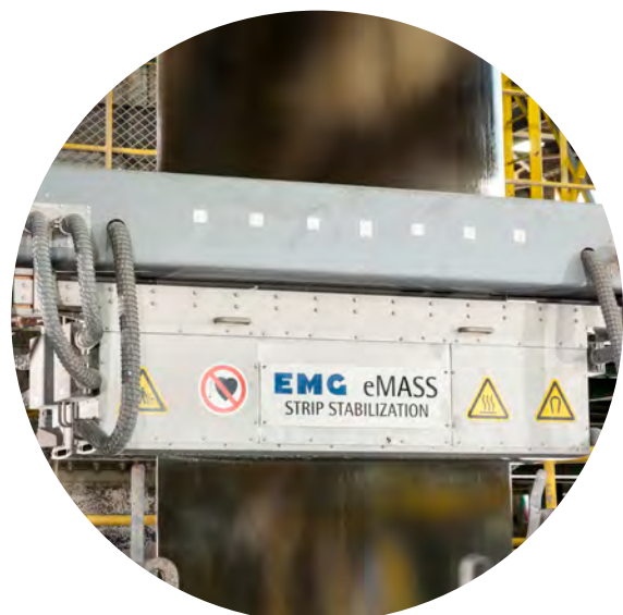
Installation on the air knife in a hot-dip galvanizing line
